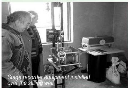
Stage recorder equipment installed over the stilling well
